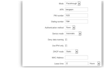
Using Passthrough Mode will disable most of the router capabilities!
