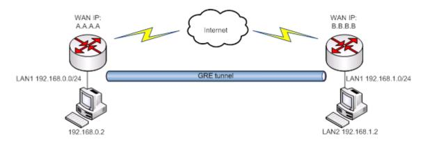
In the example network diagram two distant networks LAN1 and LAN2 are connected.
